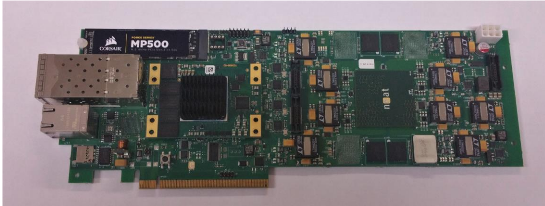
4: The EUROSERVER designed, NEAT produced, prototype board. Not shown are a Trezz 0808 module and a SIP
