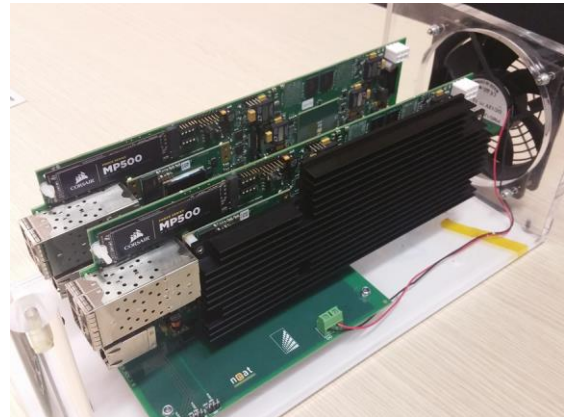
Figure 2: A pair of EUROSERVER boards, assembled onto a backplane with electrical connectivity, designed by EUROSERVER and produced by NEAT
