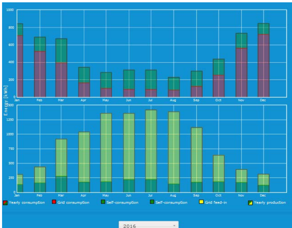
Figure 17: The figure shows in its lower part the energy production (green: self-consumption, yellow: feed into grid amounts) and in the upper part the consumption (grid: red, PV: dark green) of the year 2016 for KN10.
