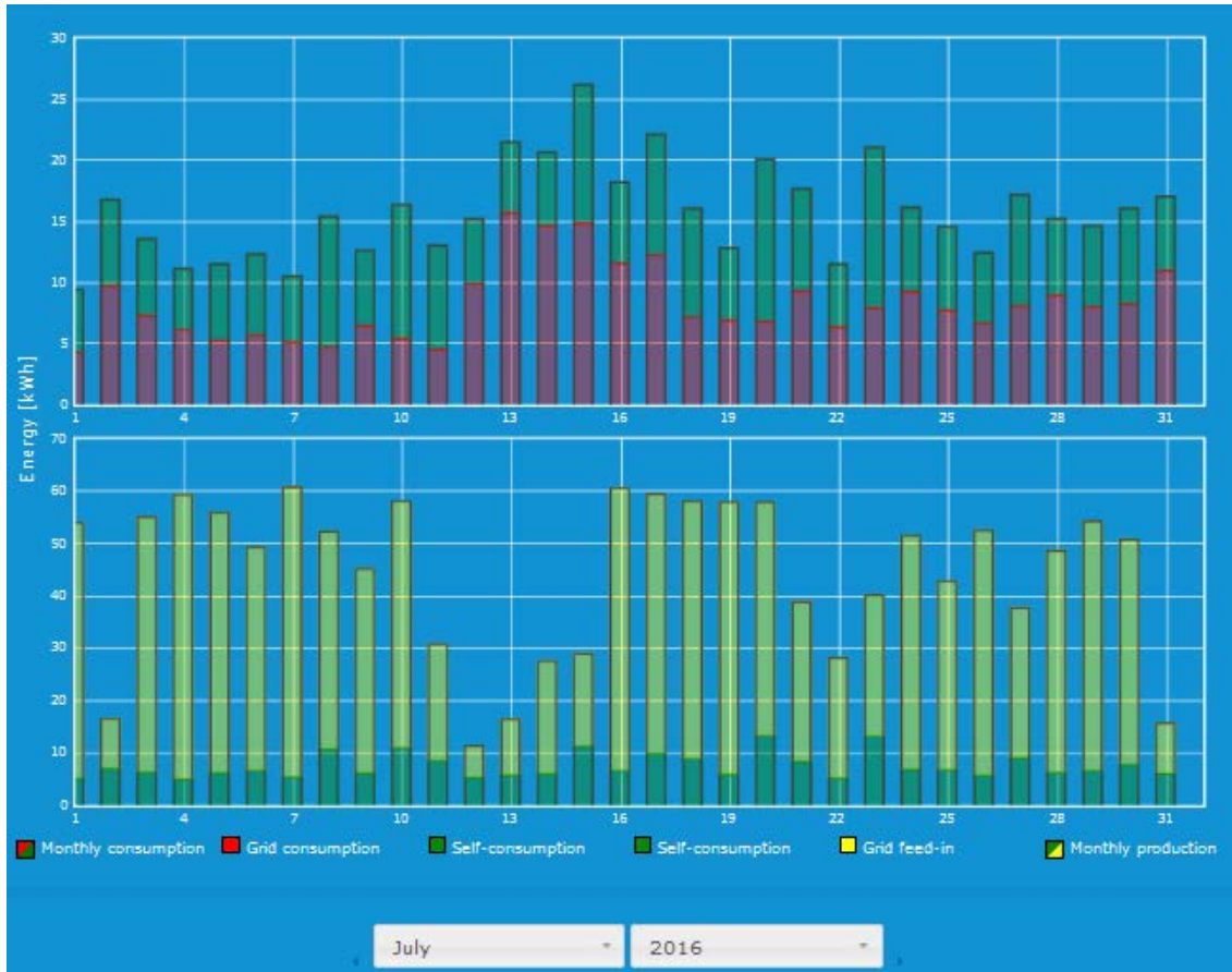
Figure 2: The bottom part shows the July 2016 PV energy production of a 10kWp PV system, in green self consumption and in yellow feed in amount, and the upper part the total consumption from the grid in red and again the self consumption in green.
