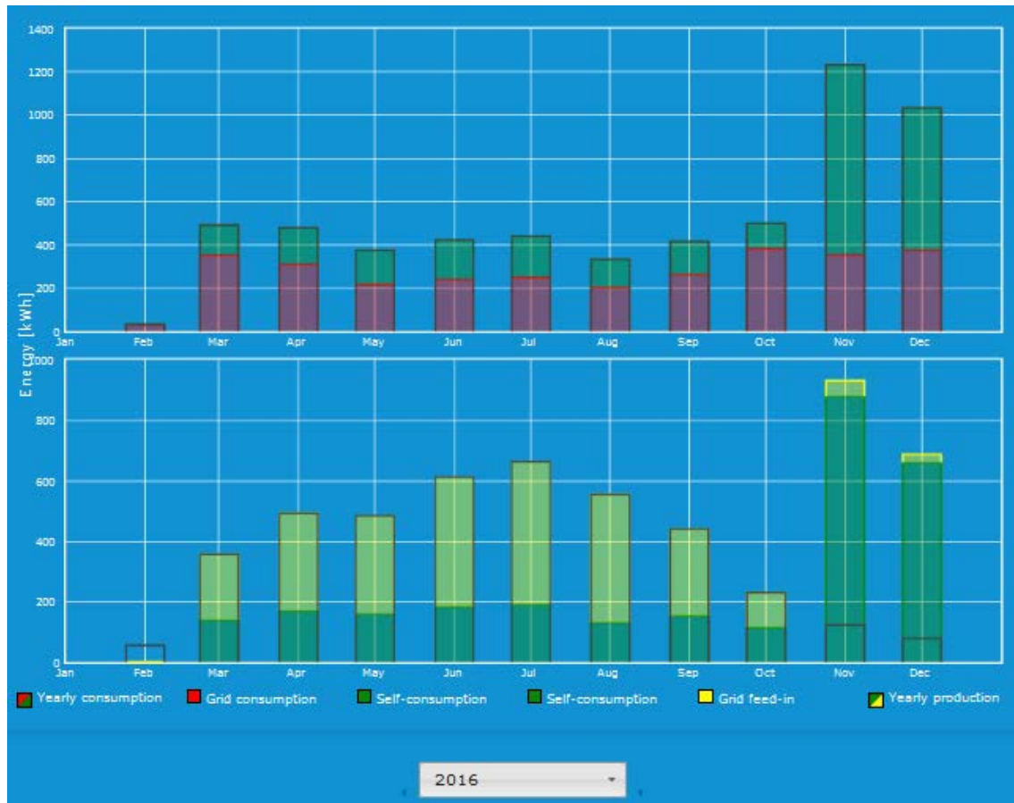
Figure 8: The PV energy production (bottom part, green self consumed, yellow fed in) and consumption (from grid in: red, and again self consumption in green) at KN09 of the year 2016. There was no data acquisition for Jan. and Feb. and serious failure in data acquisition in Nov. and Dec. for the PV generation.
