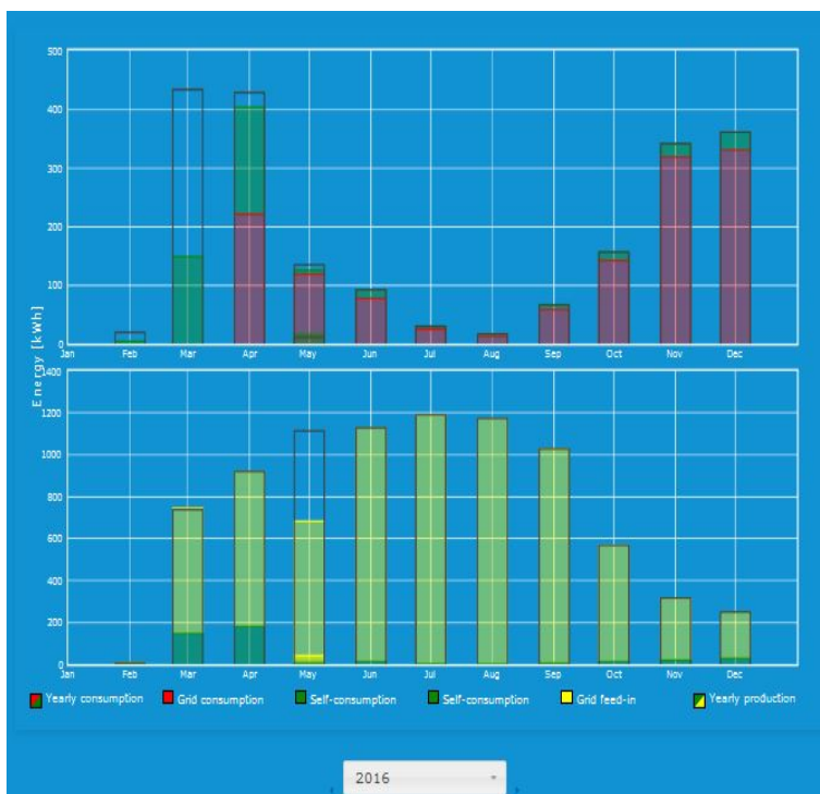
Figure 26: The PV generation (bottom, green) and the grid consumption (top, red) of KN12 shows for the time past the Tesla Power battery installation a strong reduced grid consumption. Btw there is no heat pump system installed which may cause the reduced electrical consumption in the warm half of the year.
