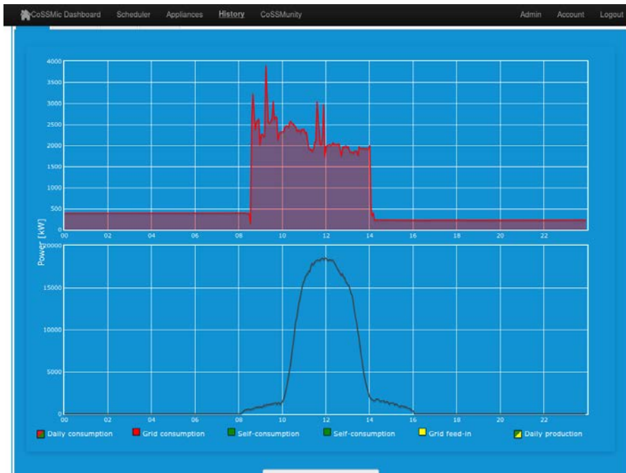
Figure 40: Daily produced (bottom) and consumed (top) power of a day in Oct. 2016.
