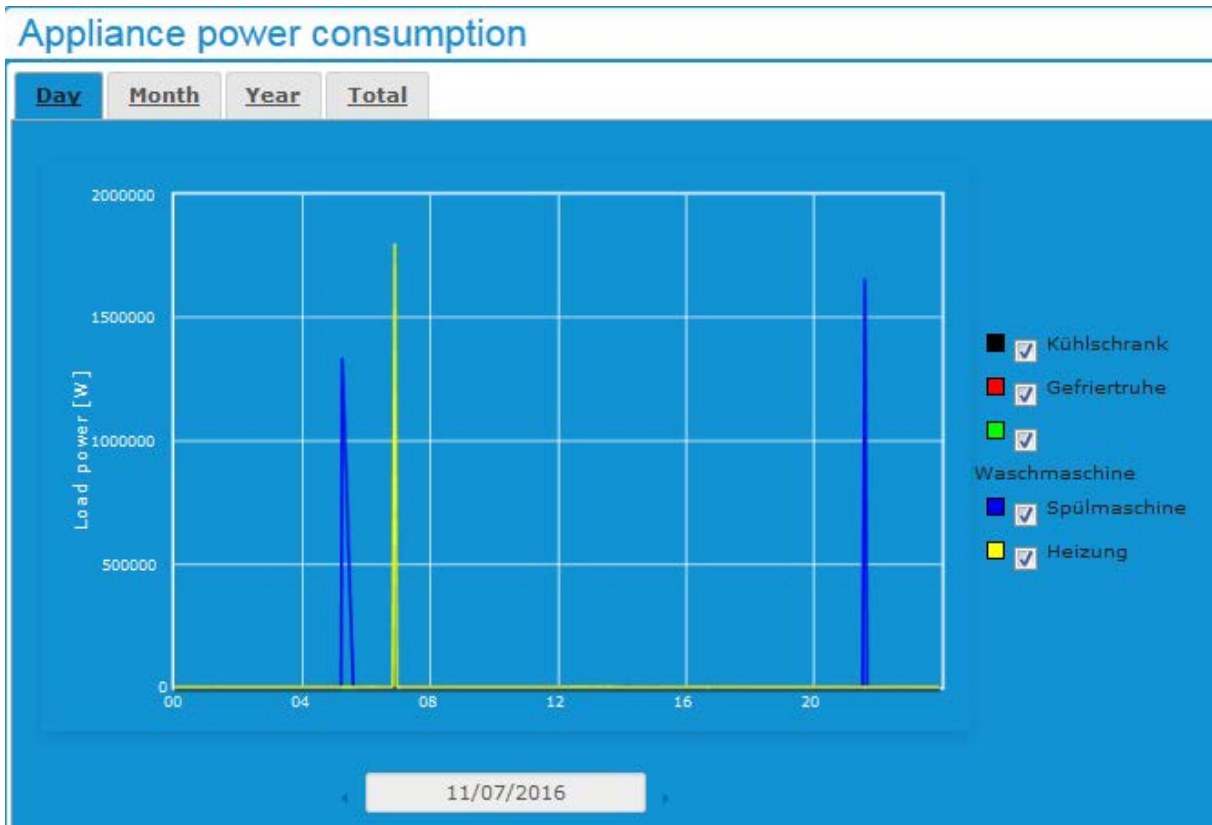
Figure 27: Displayed disturbances on the 7 th Nov. 2016 on the data branches for the pump of the heating system (i. e. Heizung) and the dishwasher (i. e. Spülmaschine).
