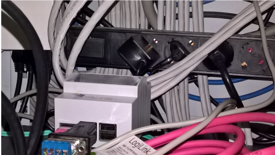
Figure 6: It shows the Raspberry PI 2 in its housing with its power supply right on top as plugged into a power socket, the red almost hidden LAN internet access behind the RS485 to USB converter in front of the picture for the data exchange between the smart meter and the Raspberry PI 2.
