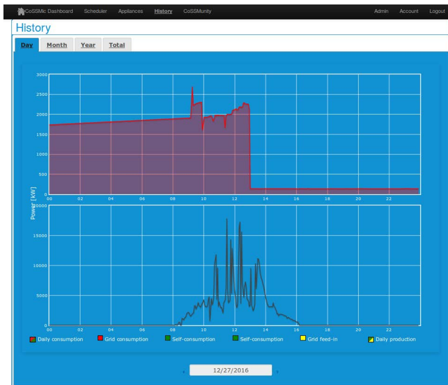
Figure 39: Comparison of consumed power and produced power by single strings.
