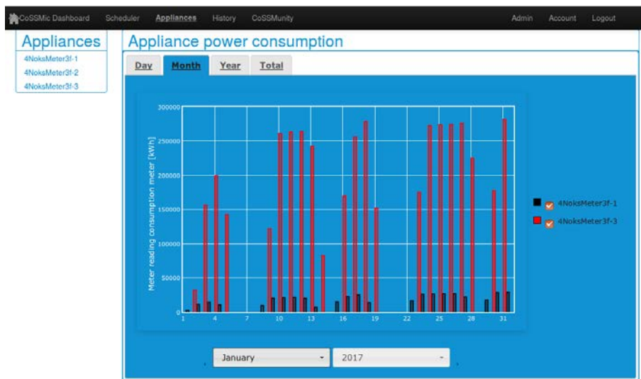
Figure 45: Monthly energy consumption measured by smart meters.
