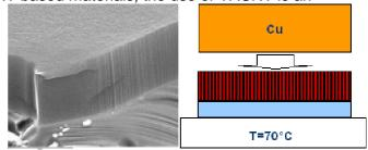
was developed in order to obtain composite like VACNT mats. The CNT assembly is brought in contact with fused paraffin (fusion temperature  $\sim$ 55°C), which spontaneously wets the CNTs. The low fusion temperature of the organic "matrix" allows the fabrication of interfaces using low temperature and pressure conditions process.
