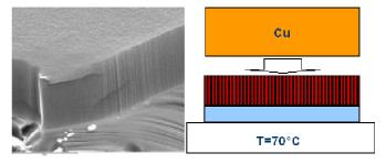
for their thermal properties. A simple method was developed in order to obtain composites like VACNT mats. The CNT assembly is brought in contact with fused paraffin (fusion temperature ~55℃), which spontaneously wets the CNTs. The low fusion temperature of the organic "matrix" allows the fabrication of interfaces using low temperature and pressure conditions process.
