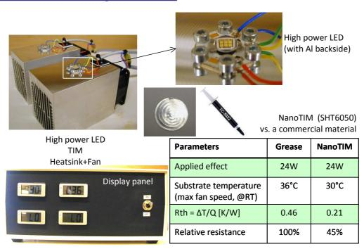
NanoTIM, a metal-polymer composite material whose development is leaded by Chalmers University in the framework of the NANOPACK project, has been applied as TIM in the assembly of high power LEDs.
