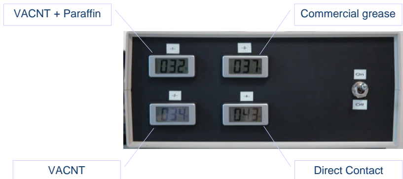
Monitoring the T° of the 4 LED
