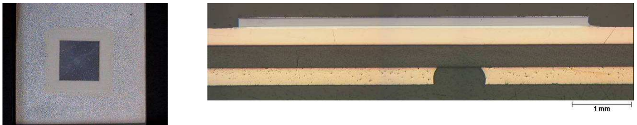
Figure 1: Left: Light microscopy image, top view of the chip sintered on DCB; Right: Cross section of a Ag-sintered Si chip on DCB
