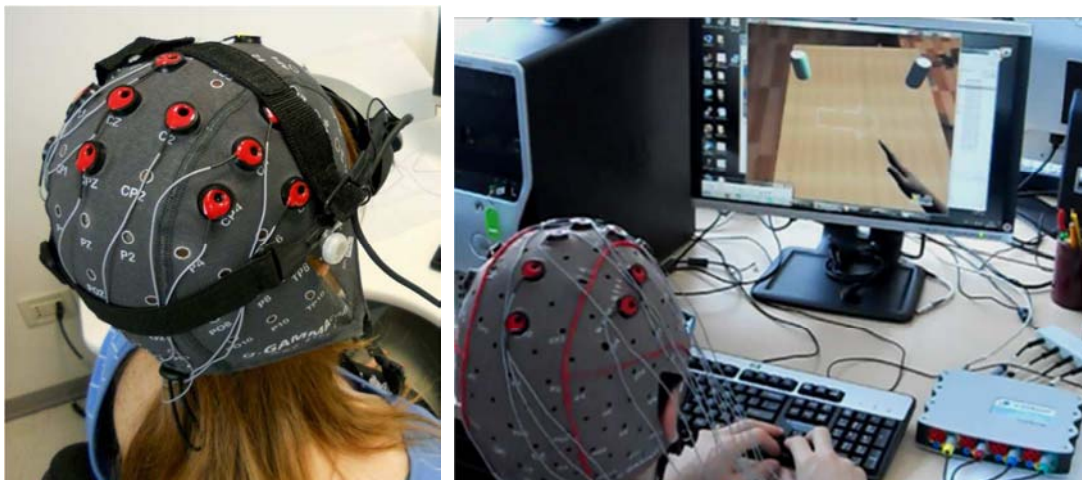
Figure 10 The EEG brain computer interface based on motor imagery, here shown for the virtual embodiment condition.
