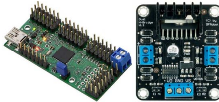
Figure 7 Overview of the micro-controller board (Pololu Micromaestro) and h-bridges ICs implemented into the Tactile Vest
