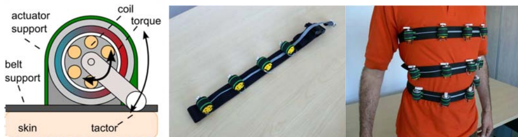
Figure 6 Detail of the tactile vest actuators and Tactile vest modules worn onto the user's torso
