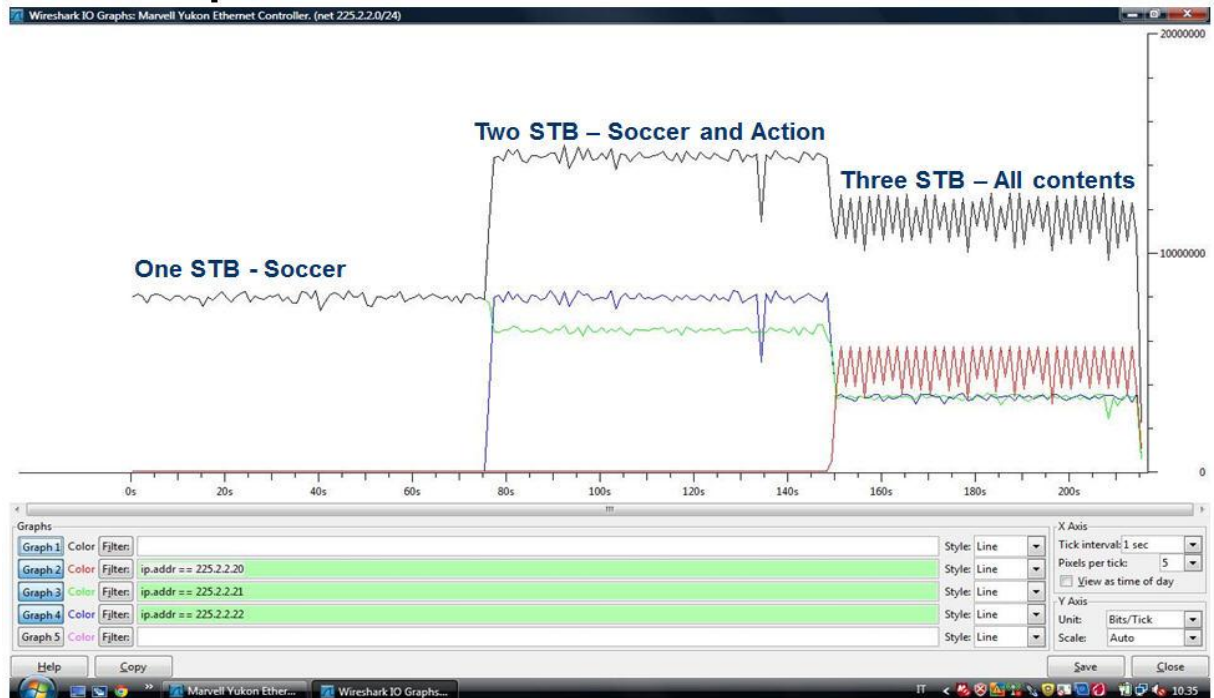
Figure 11: Wireshark acquisition of the used bandwidth by the 3 TV-SETs
