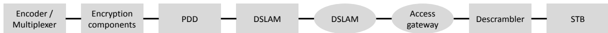
Figure 20 General view of the test setup (square elements are the ones specific to the OptiBand project)
