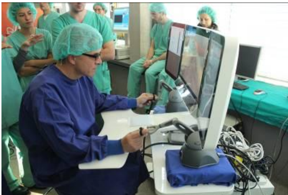
Figure 8: Training in operating the SPRINT. The surgeon is using two master arms for guiding the SPRINT slave arms.
