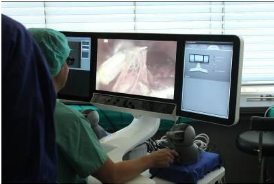
Figure 9: Training in operating the SPRINT: view point of the surgeon. A central video screen offers 3D vision, two lateral displays provide ancillary information about the system.
