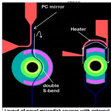
Layout of novel microdisk sources with external cavity controlling wavelength and directionality
