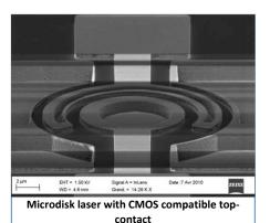
compatible with 9GBit/s data transmission. The results of these initial experiments where then transferred to the 200mm processing line and we demonstrated for the first time operational III-V microdisk devices fully processed in a CMOScompatible line, on a 200mm wafer. Using a
