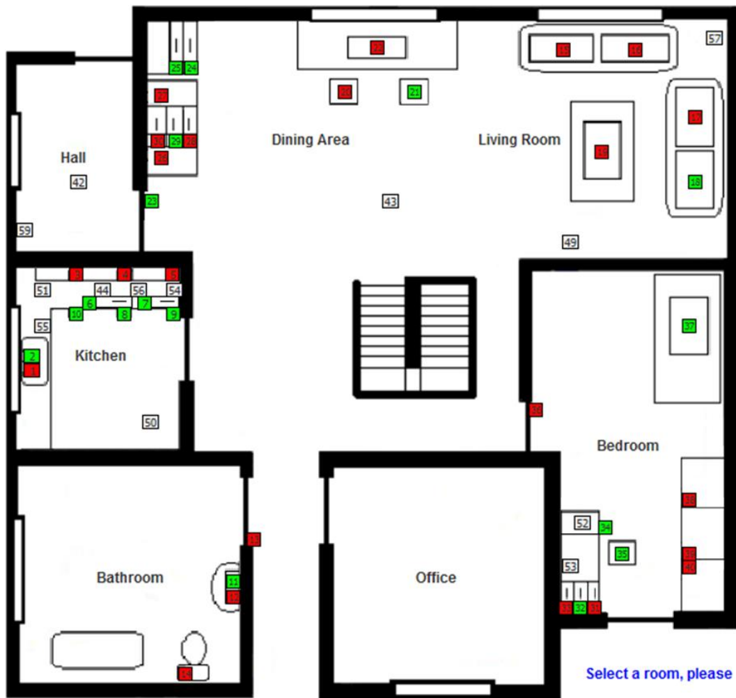
Figure 1 - UH Robot House map showing the location of sensors (identified by numbers) and their states with green colour representing the sensor in open/on/free state, red colour representing the sensor in close/off/occupied state and transparent representing the sensor is not activated/unknown.
