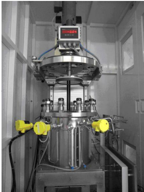
Figure 5: The prototype: a) autoclave system; b) mixing tank
