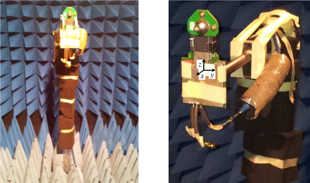
Figure 37 : Experimental setup for the measurement of the isolated sensor in anechoic chamber.
