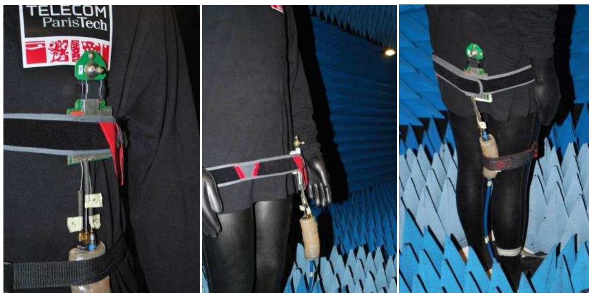
Figure 51 : Sensor positioning on the phantom: left chest, left hip and right back.
