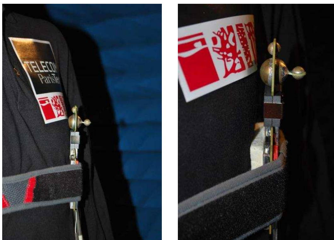
Figure 52 : Sensor/phantom spacing: ~ 0, 10 and 20 mm (not shown here).
