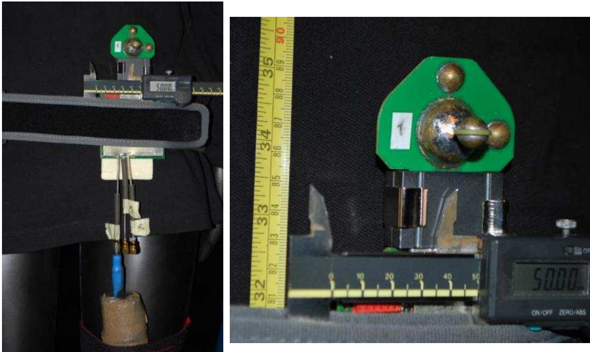
Figure 55 : Sensor positioning details: right back, ~5 cm from the saggital plane and ~ 87 cm from the ground.
