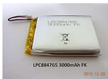
Figure 35 : Flat battery identified for the LEXNET dosimeter
