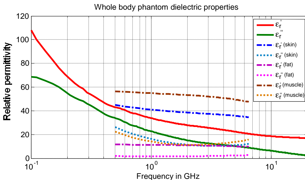
Figure 49 : Whole body phantom (“Kevin”) dielectric properties (from [17]).
