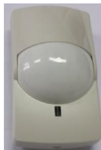
Figure 5. Presence sensor. It must be strategically placed in the home to properly capture the primary user movements.
