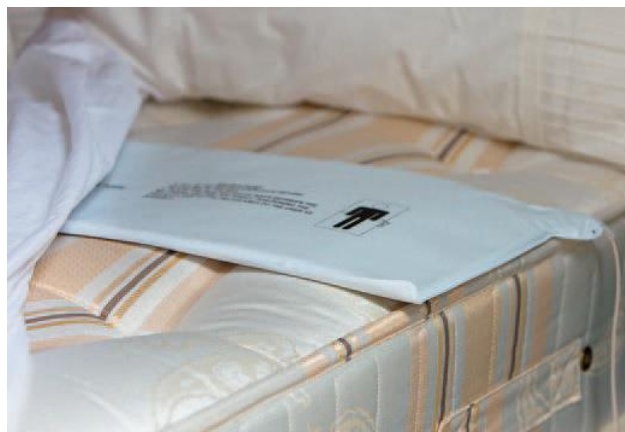
Figure 7. Occupancy sensor. This pad requires an universal sensor to wirelessly transmit the information.
