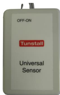
Figure 9. Universal sensor. It permits any compatible device to wirelessly communicate to the GiraffPlus middleware.
