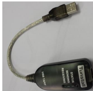
Figure 4. USB Tapit. This device permits the connection of the Lifeline Vi+ unit to a computer.
