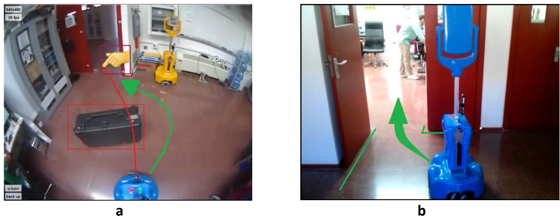
Figure 17 Two typical cases where the collaborative control proves its suitability for teleoperation. a) The user drives the robot towards an obstacle. b) The user wants to cross a door by marking a point inside the room. In both cases the collaborative control generates appropriate paths to arrive the user destination while negotiating obstacles.
