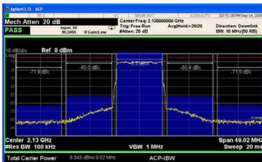
Figure 2.24: ACLR in commercial HPA (+10dBm over 10MHz)
