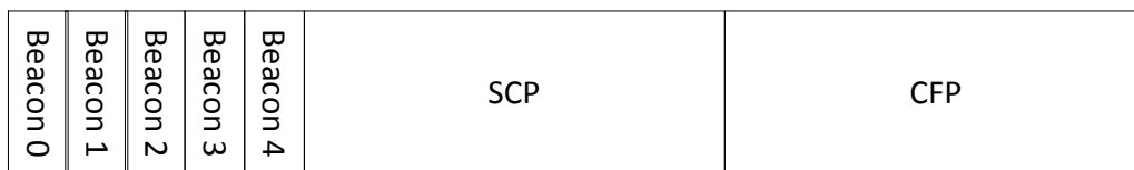
Figure 4: PRIME MAC superframe structure [6]
