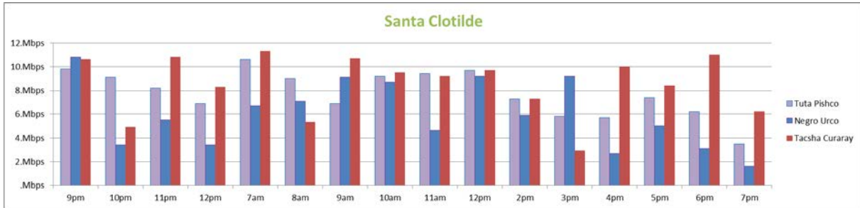
Figure 58: Measurement of the bandwidth available from Santa Clotilde using the bandwidth-test tool
