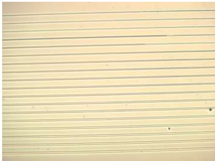
Figure 3: Optical microscopy image of an array of waveguides etched to a depth of 4.8 mm, of widths between 1.5 mm (top of image) and 10 mm (lower part of image), fabricated by plasma etching using chlorine-based etch chemistry
