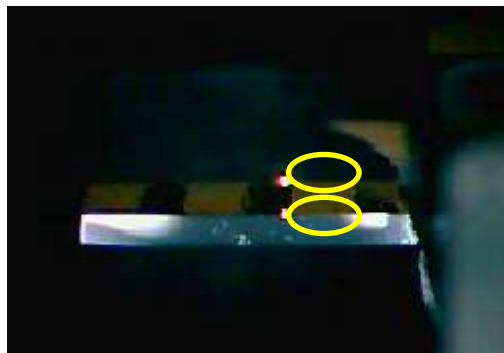
Figure 2: Observation of wave guiding. The camera was tilted so that the light entering the waveguide can be seen in the upper circle whereas the transmitted light can be observed in the lower circle.
