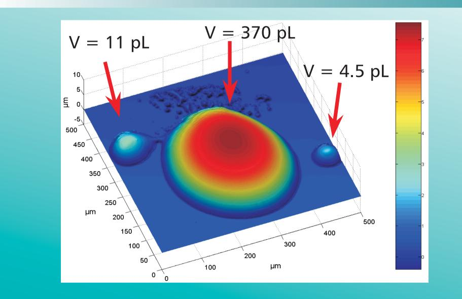
To determine the concentration of organic substances carried by the droplets, the shape of the droplet is determined by optical interference spectroscopy. The optical system is combined with a nanopositioning system enableing a spatial resolution of 200 nm.
