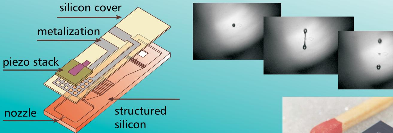
Inkjet like dosing system for nano- and pico droplets of water based liquids. The system provides droplets with volumes between 1 and 50 pL, a spatial precission of
