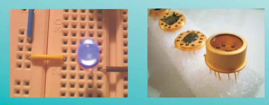
To identify organic substances embedded by the droplets optical spectroscopy is requried. InGaN/GaN heterostructures are processed into optical emitters and detectors sensitive only in a narrow spectral range. This range can be tuned through the visible and near UV.
