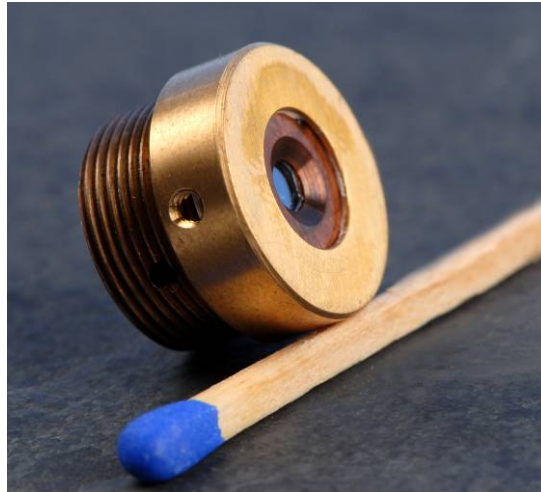
Core of the VERTIGO laser technology: the semiconductor gain chip for the 2 – 3 \mu\text{m} wavelength range embedded in a custom designed heatsink.
