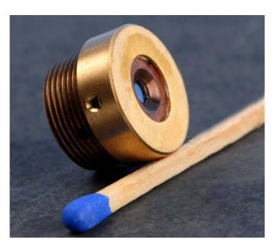
Core of the VERTIGO laser technology: the semiconductor gain chip for the 2 – 3  $\mu m$  wavelength range embedded in a custom designed heatsink. Foto © Fraunhofer IAF
