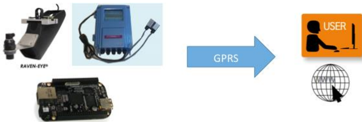
Figure 6-6: How Ultrasonic flow meters and BBB work together
