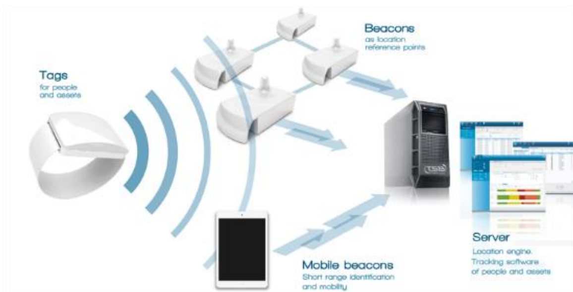
Figure 18 MYSHERA RTLS working diagram
