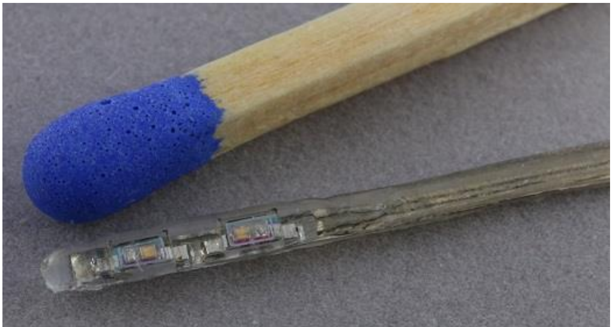
Figure 7: Long term implantable optical electrode for optoacoustic sound enhancement. The implant contains two hermetically packaged VCSELs (see Figure 6Error! Reference source not found.), which are oulded in silicone. The device is 10 cm long. Only the distal end is shown. The match is for size comparison.
