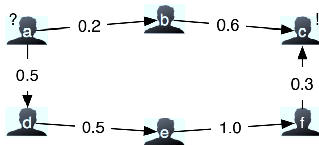
Figure 12 A simple propagation example with two paths from the truster to the trustee
