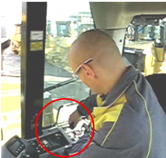
Figure 20: Connecting ET tool to ECM
