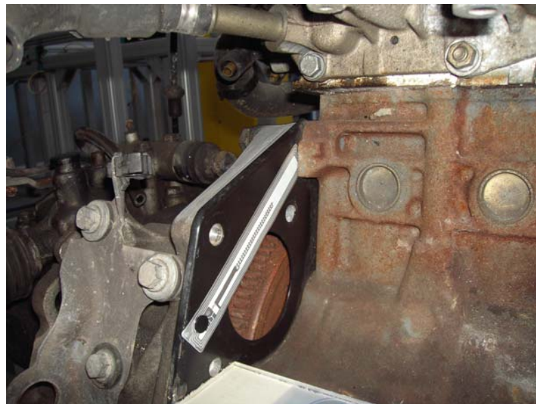
Figure 2. The tag on the clutch’s housing
