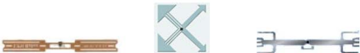
Figure 2: Different forms of passive tags (source: Emerson & Cuming, www.eccosorb.com/rfid )
