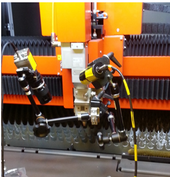
Figure 11: The experimental set-up of the HSI camera and illumination laser, before alignment, in the laser cutting workstation.
