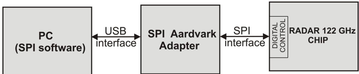
Figure 9 PC, Aardvark Adapter and Radar 122 GHz chip
