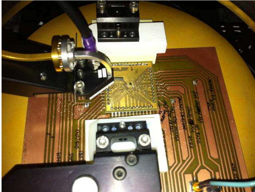
Figure 30. Probe station setup, the 122GHz interface is directly probed on-chip.
